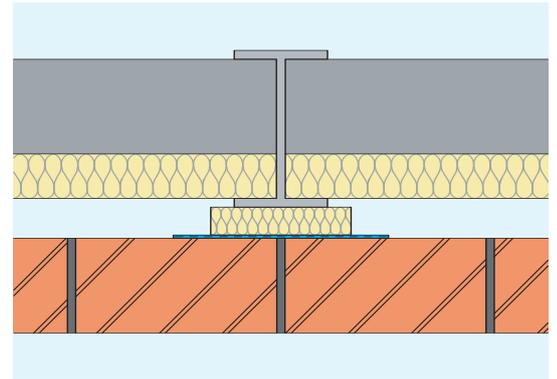
Figure 5 Plan view of steel frame construction with Rockclose
