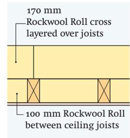
Figure 1 Cross layered roll U value 0.16W/m<sup>2</sup>
